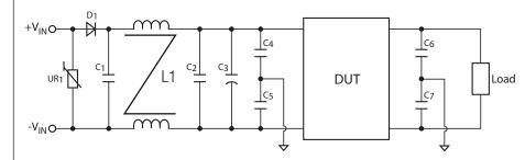
It is recommended to add UR1, D1 and C1 in railway application. C1, L1, C2 and C3 can be modified for required EMI standards. To meet EN61000-4-2, module case should be earth grounded. We offer independent case pin option on request.
