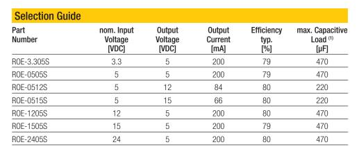
The ROE DC/DC converters are typically used in general purpose power isolation and voltage
